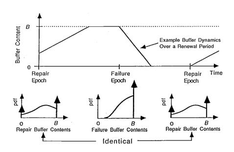
Case 1: Speed 1 > Speed 2 and buffer partially full at repair, buffer fills before next failure, next failure is Station 1, and buffer empties before repair.
