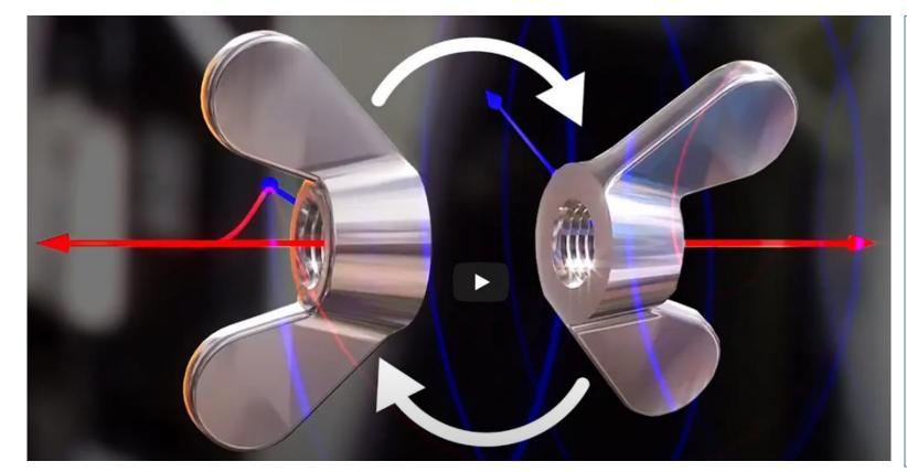
The Dzhanibekov effect – a special case of the free rigid body motion spinning around the *middle* axis of momentum of inertia. An instability of spin around the middle axis has been known since the 19th century.
