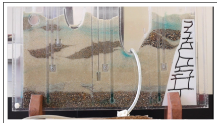
Figure 2: Sand Tank Groundwater Model.
