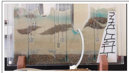
Figure 2: Sand Tank Groundwater Model.
