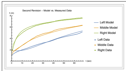
Figure 9: Second Revision: Variable Head Level at Right Boundary and Variable Initial Head Level.
