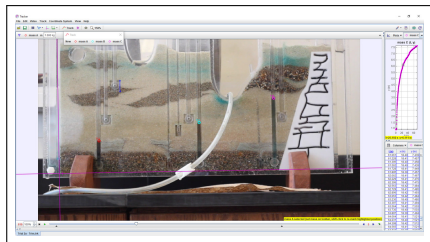
Figure 4: Collecting Well Head Data via Tracker.
