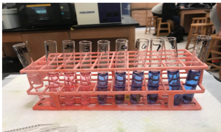
Figure 18.2: Figure 1 shows the difference in color for test tubes 1-3 which had pH 3 buffer, along with the same constants the rest of the tubes had. This photo shows why the procedure deviation was necessary.
