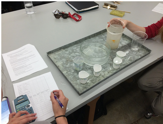
Figure 1. General set-up of the Lesson. This figure shows the equipment used for the experiments. A large tray contains a 1000 ml beaker and a student is holding a 500 ml clear cups with holes over it. There is also a 500 ml clear cup without holes, large bowl with water and a 50 ml plastic beaker, four 120 ml (4 ounce) paper cups, and one 200 ml (7 ounce) paper cup. Another student is filling out a data sheet.
