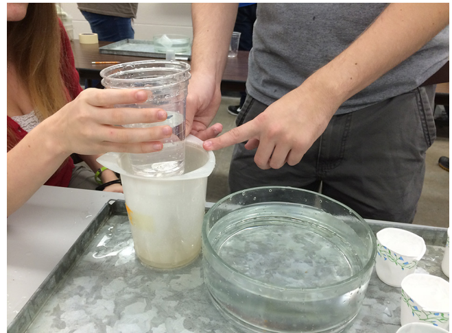
Figure 3. Stopping the trial. This figure illustrates how a trial is stopped. To stop a trial and stop the leakage, the clear cup without holes is quickly placed under the cup with holes.
