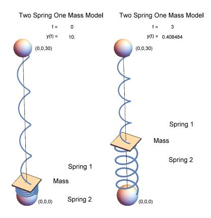
Figure 1. Two springs with fixed ends and one mass in two positions. On the left the view is when the spring system is in static equilibrium, i.e. at rest, while on the right is when the mass is displaced vertically down from static equilibrium.
